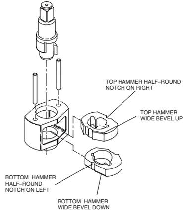
1. Coat the Hammers (39) with a light film of Ingersoll Rand No. 170 Grease.
