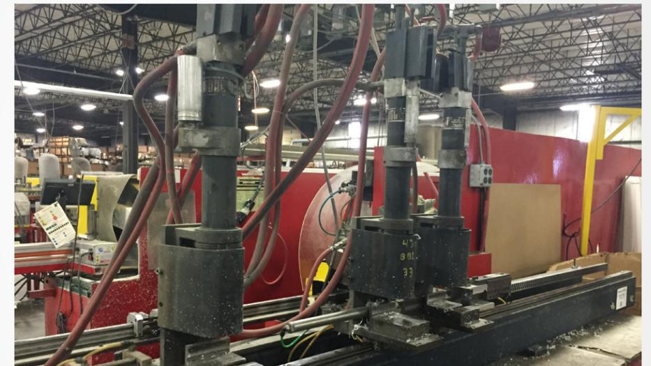
minimizes tool size and weight for added machine design flexibility. The tools are easy-to-install and require only simple pneumatic circuitry.
