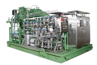
Two-stage MSG-11 operating as a debutanizer compressor in an NGL fractionation plant
