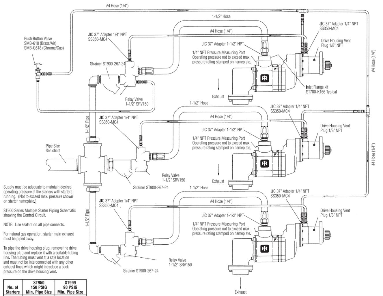
Supply must be adequate to maintain desired operating pressure at the starters with starters running. (Not to exceed max. pressure shown on starter nameplate.)
