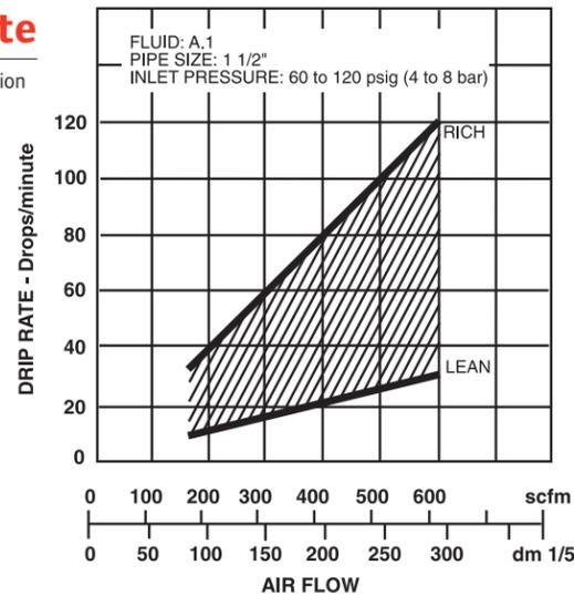
FIGURE 1 Recommended Drip Rate Settings for Average Lubrication
