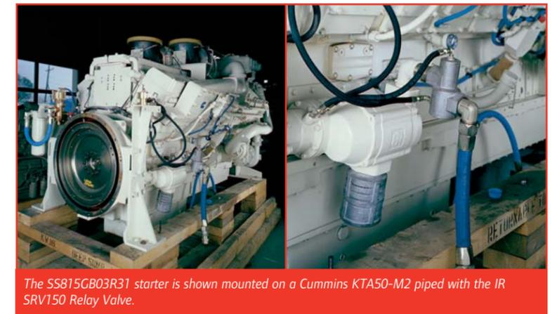
The SS815GB03R31 starter is shown mounted on a Cummins KTA50-M2 piped with the IR SRV150 Relay Valve.
