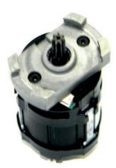
1. Install the motor mount onto the motor. Align the mount so that the slot in the mount is on the opposite side of the motor from the motor connector as shown in the photo. Torque the motor mount screws to 0.5 Nm.
