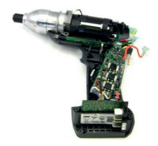
15. Install the Handle PCB onto the center screw lug. Ensure that the O-ring is in position on the lug underneath the board. Again ensure that all the cables are routed properly and fully seated.
