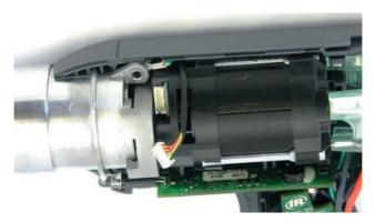
14. Connect the Hall Cable with its connector on the motor.
