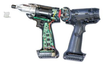
4. Carefully remove the housing clamshell ensuring that you do not damage any of the cables or connectors.
