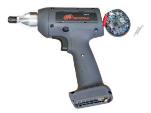
22. Install the backcap onto the housing and secure it with two screws tightened to 1 Nm.
