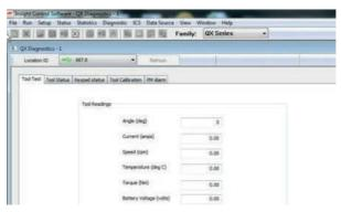
7. Next select the Diagnostics tab on the menu bar. Then select System Diagnostics from the drop down menu. Examine the settings under the Tool Test, Tool Status, and PM Alarms tabs for any unusual settings.
