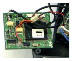
10. Connect the Hall Cable to its connector on the foot PCB, the transducer cable to its connection, and the connection between the foot PCB and the handle PCB.
