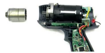
9. If the Gear Pack has remained on the motor, remove it from the motor, and set aside. We will disassemble this later in the program.
