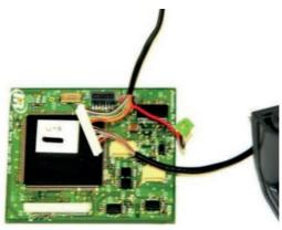
9. Connect the connector of the Interface cable to its connector on the foot PCB.
