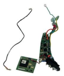
16. This will leave the Hall Cable which can now be disconnected from the foot board and the cable removed.
