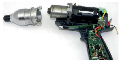
8. Tilt the motor and gear case assembly up at a slight angle, then carefully remove the gear case assembly from the motor.
