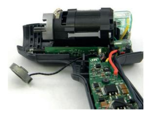
$10. \ While \ tilting \ the \ motor \ up \ slightly, \ remove \ the \ transducer \ from \ the \ front \ of \ the \ motor.$
