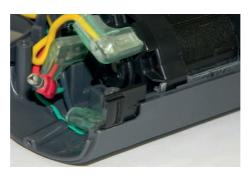
17. Install the USB port cover into its slot.
