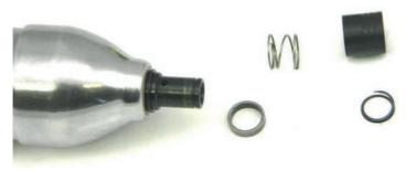
1. For units with the ¼" quick change spindle, disassemble the spindle as follows. Remove the spiral spring clip from the front of the spindle, then remove the quick change collar, spring, spring support and rear spiral snap ring.
