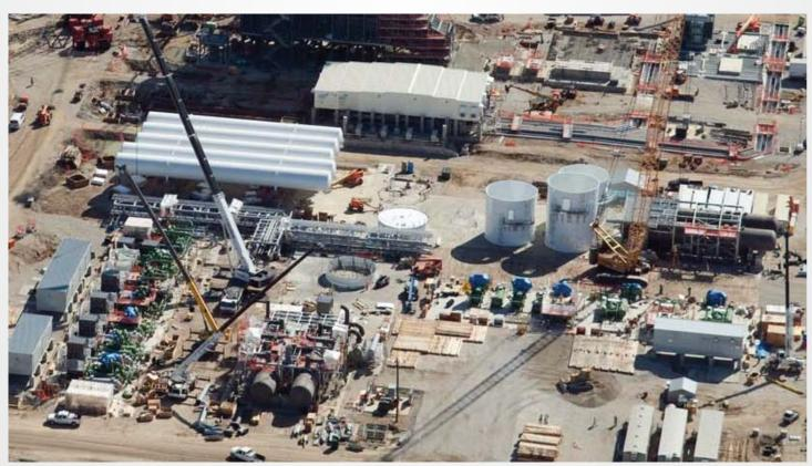
Work site for construction of an IGCC power plant in the US. Ingersoll Rand field service technicians were on site to coordinate the installation and commissi of thirteen MSG-16 compressors.
