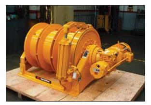
Custom launch vehicle payload handling winch
