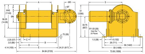
Note: Dimensions are for standard base models only and subject to change. For optional drum lengths and gearbox combinations please contact the factory for dimensional drawings.
