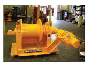
21,300 pound maintenance winch with dual brakes and vector duty motor
