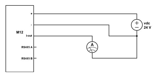
The current meter is placed in between the current output and the power supply ground. You can also use a digital multi meter to test the current output.
