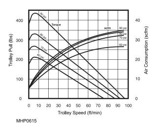
Figure 2. Performance based on 90 psig at the motor inlet  $\,$
