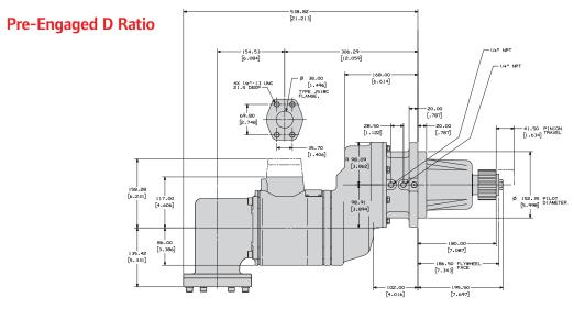
Note: Illustrations not to scale. Dimensions in mm (in). Elbow exhaust shown for pre-engaged models, but straight exhaust is also available. Elbow exhaust configuration is also available for the inertia starter shown above.
