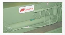
All MSG TURBO-AIR compressors feature a self-contained, low-pressure lubrication system.
