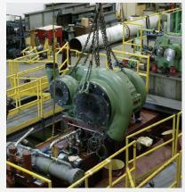
Multi-stage carbon monoxide compressor being prepared for closed-loop testing
