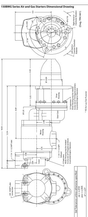
Starters should be installed on the Engine with the exhaust pointed down.
